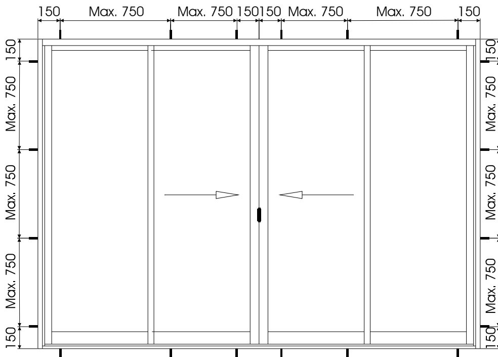
TYPICAL OXXO SLIDING DOOR & HORIZONTAL SLIDING WINDOW
